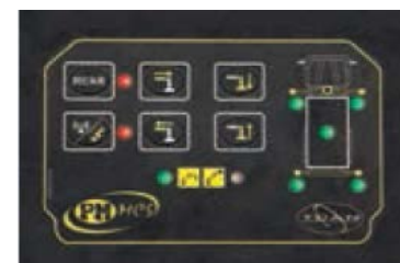
Remote controlled outriggers and MCS system
